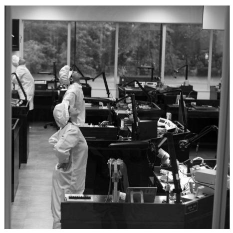
On the same floor as the machine assembly of cheap watches, a small team of skilled workers assembles mechanical Grand Seiko–model watches by hand. The team (seen here during one of the compulsory exercise breaks) makes about a hundred watches a day, using components that are all, from hands to hairsprings, made in Japan, also by Seiko.
