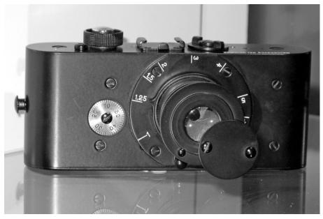
The prototype Ur-Leica, fashioned in 1913 by the Leitz employee Oskar Barnack. It was small, light, with a near-silent shutter, and a  $24 \times 36$  mm film format.
