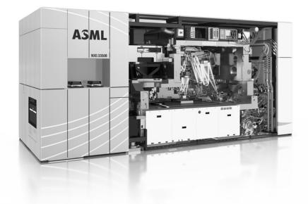
It takes an enormous machine to allow for the making of something so infinitesimally tiny as a computer chip. This Twinscan NXE:3350B photolithography machine, made by the Dutch company ASML, would fill three jet cargo aircraft. Intel, the world's biggest chip maker, buys these \$100 million machines by the score.
