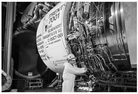
Despite the apparent fantastical complexity of a modern jet engine—here a Rolls-Royce Trent, four of which power the enormous Airbus A380 double-decker superjumbo jets—there is essentially only one moving part, a rotor that passes through the entire length of the engine, from fan to exhaust.
