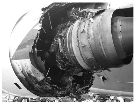
The wholly destroyed Rolls-Royce Trent number two engine after the safe landing in Singapore of Qantas Flight 32 following an "uncontained rotor
