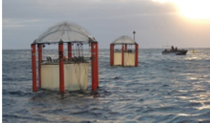
KOSMOS mesocosms in Gran Canaria, used to study the effects of increasing acidity on open ocean ecosystems
