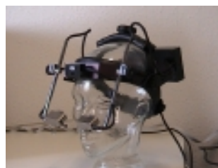
Figure 2.1: Mounted helmet for eye-tracking experiments.
